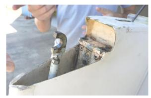
fuselage, use the bungee cord to prevent it from moving (if the control connection is left facing outward it can damage the wing).
