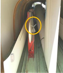
13) Flip up ramp and close trailer up. Before closing front of trailer check that the spoilers are in.
