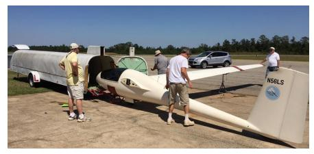
trailer and slide in. The wing dolly wheel is on the lateral side of the cart track! This wheel needs to come to rest in the matching depression in the trailer floor (otherwise trailer won't close later). At front of trailer check that the pin on the wing protrudes through the holding device on trailer. Use small wing nut to secure wing root to holding device. Foam pipe insulation pads get stuffed around the control rods so they don't flap around during transport.
