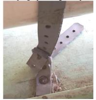
12) Place rack with horizontal on left side of fuselage and secure with threaded bolt. (Reminder the Horizontal's metal T control fitting must face inward)
