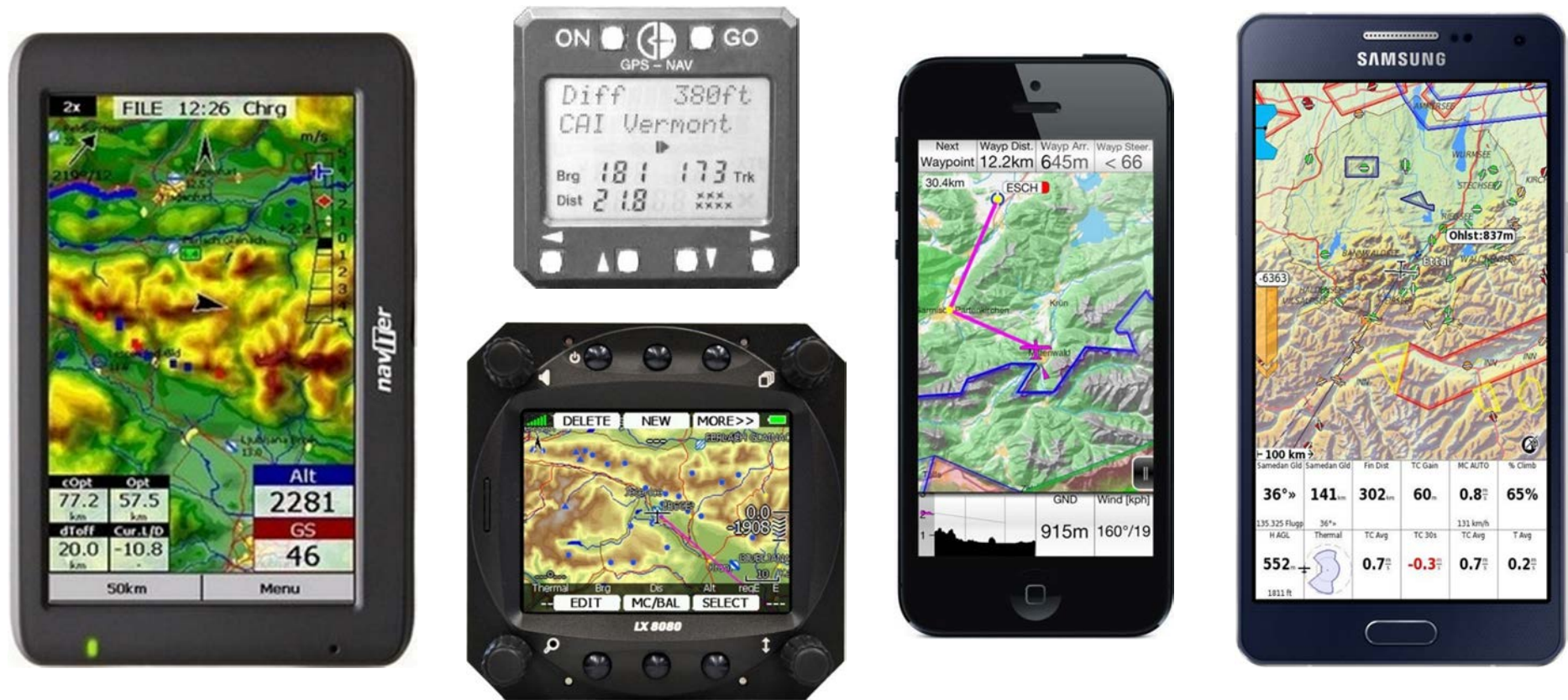
From left to right: Oudie, Cambridge 303 (top), LX 8080 (bottom), iPhone running iGlide, Android smartphone running XCSoar (shown approximately to scale)
