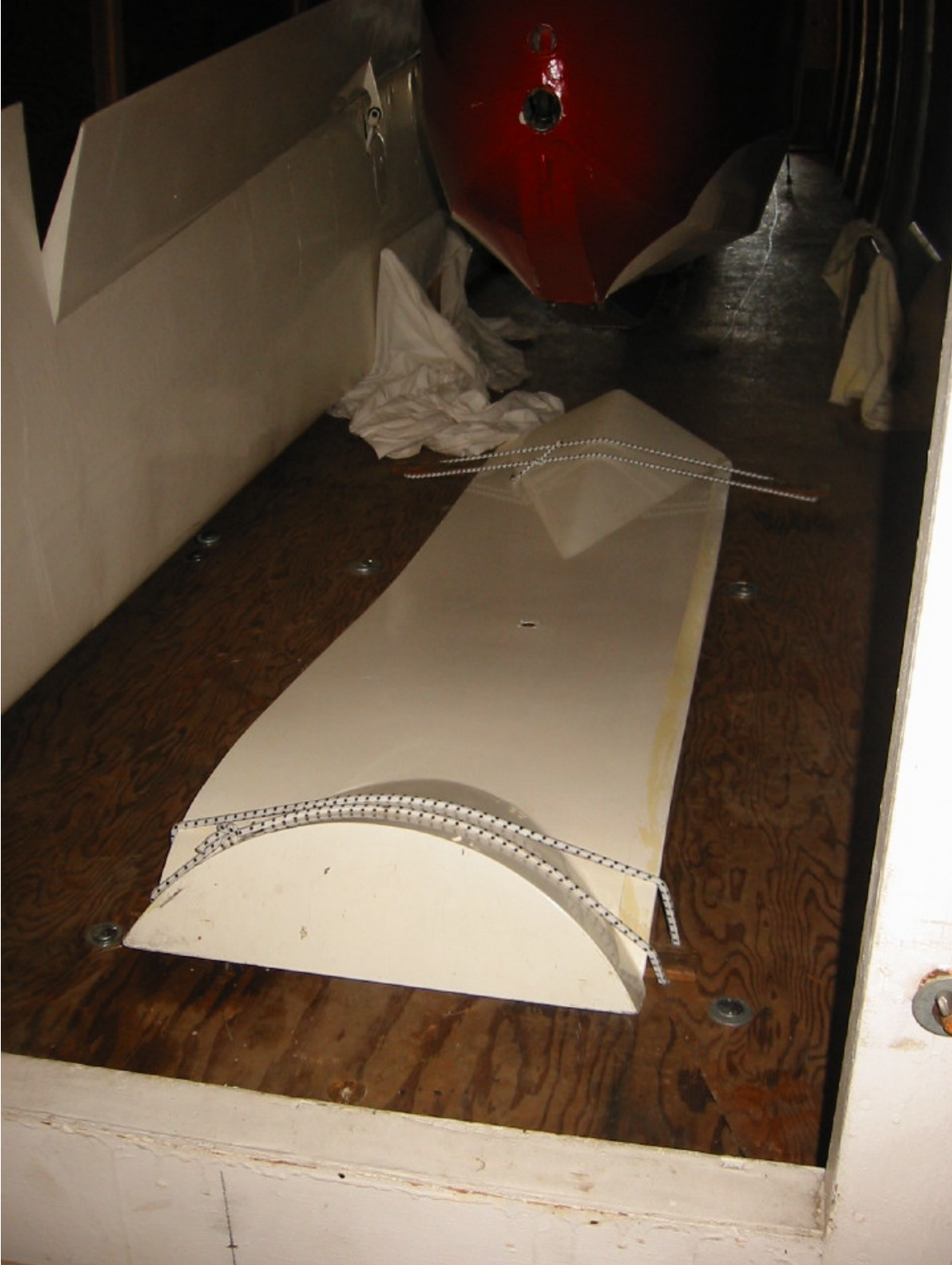
Photo 8. Turtle Deck Secured to Trailer Floor. Note: Antenna may need to be removed. (Photo does not show Left Wing Alleron lock)
