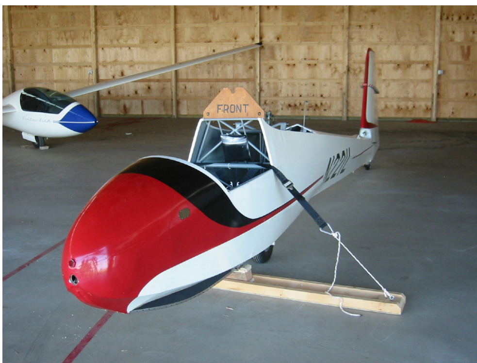
Photo 4. Fuselage on Stand ready to be Inserted into Trailer. Note: Attach Canopy after Removing Stand.
