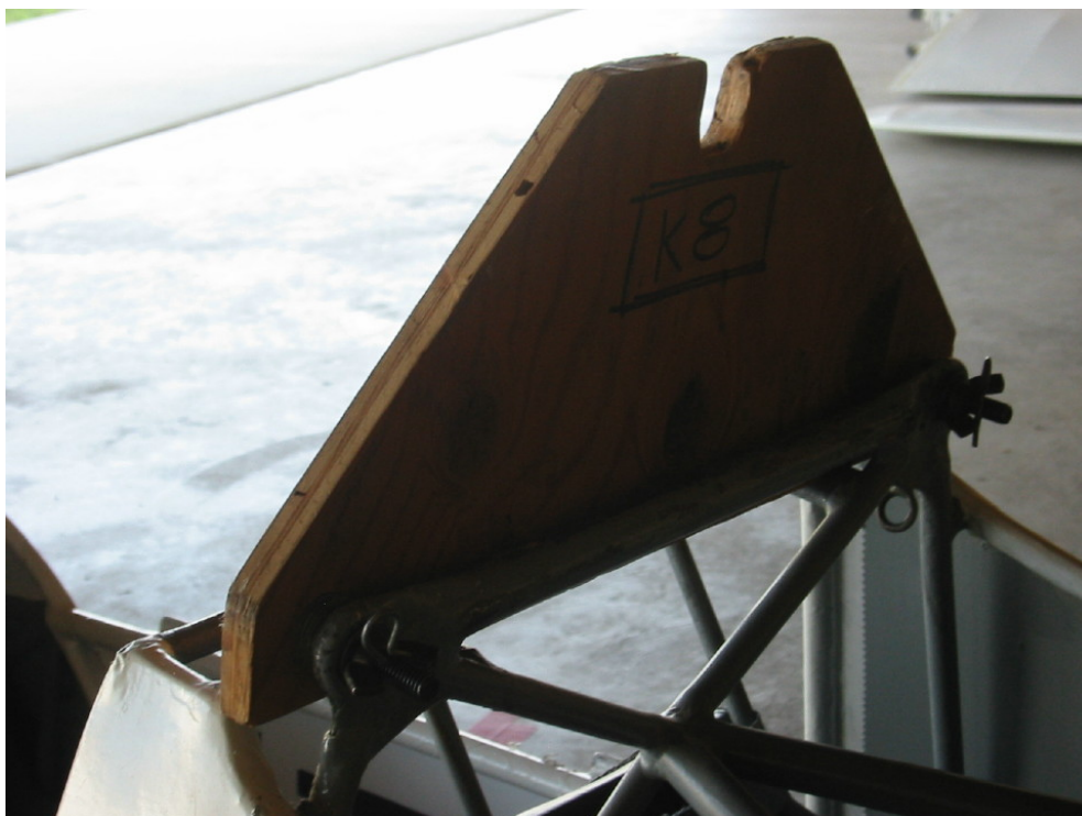
Photo 3. Carriage Guide attached to Fuselage with Wing Nuts and Safeties.
