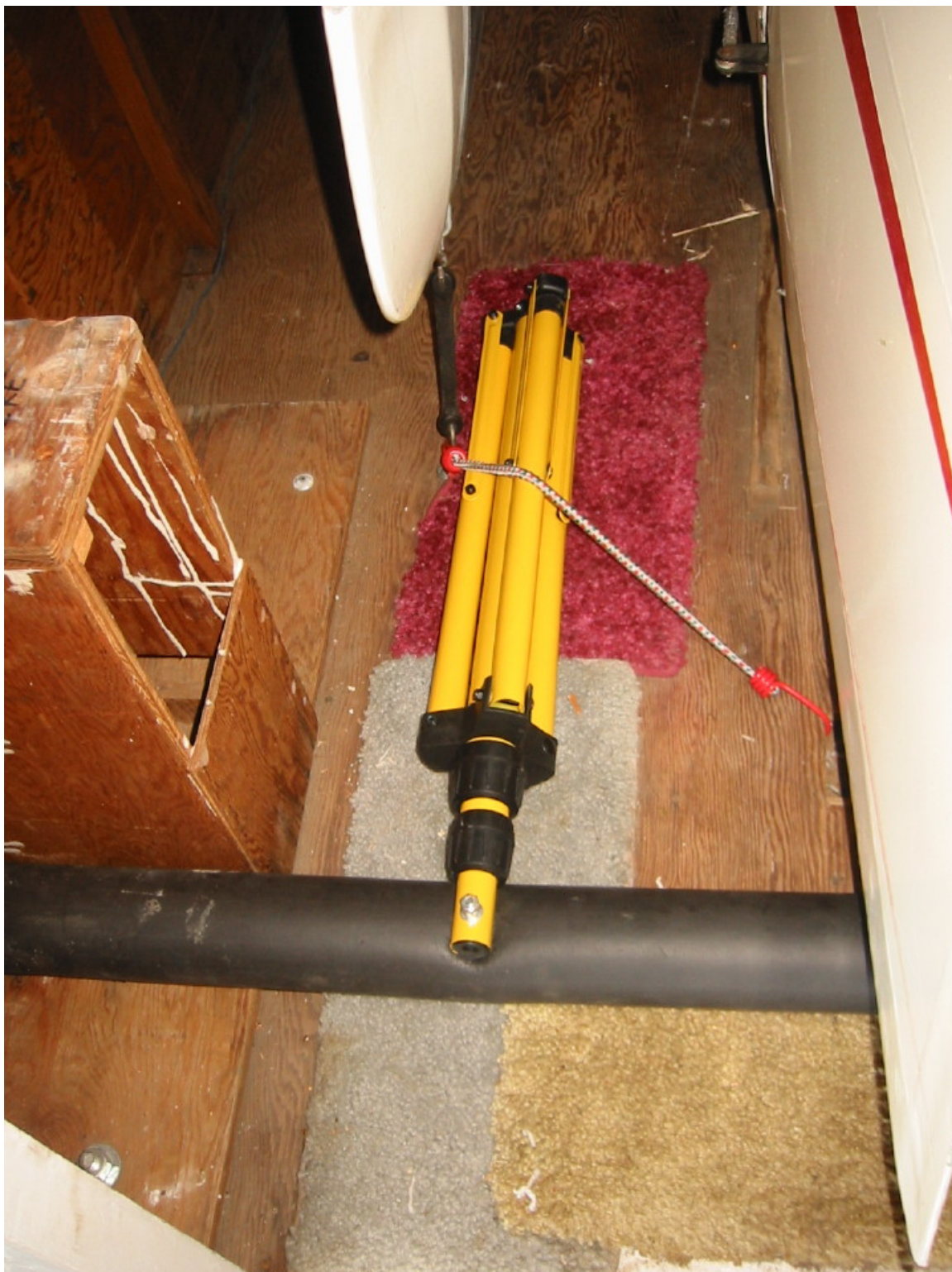
Photo 9. Wing Stand Secured to left rear Trailer floor.
